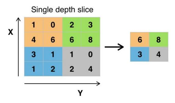
Max-pooling is when you add a pooling layer, causing an image is separated into non-overlapping rectangles, with each sub-region's maximum being outputted afterwards. This reduces the spatial size of the image, controlling overfitting by reducing the parameters and computation needed to interpret the image.
