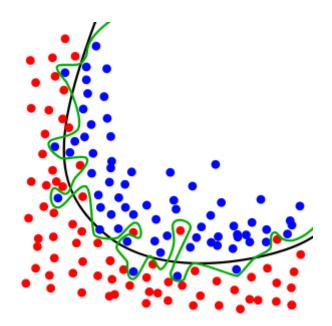
An example of overfitted data. The black line is nicely fitted, while the green line tried too hard to be 100% accurate. But if other data will be inputted, the error will increase.
